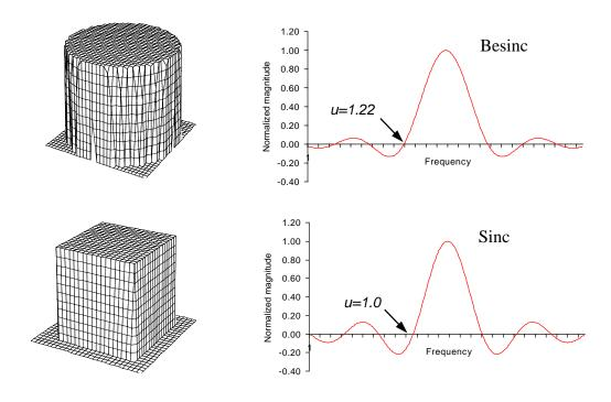
Figure 1 Circular and square shaped pupils and their corresponding transforms.
