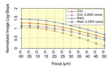
Figure 11. Effects of coma on NILS for circular and square (rectangular) source shapes.
