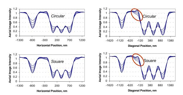
**Figure 6.** 2D image comparisons for a horizontal cut-line through elbow pattern for circular and square source shapes.
