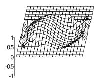
**Figure 10** Impact of illumination on coma aberration effects. The diffraction field is plotted for  $k_1$ =0.38 with  $\sigma$  = 0.7 and 0.25 waves of primary coma.
