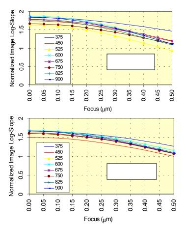
**Figure 14** Annular vs. square ring performance measured as NILS through focus and pitch. Wavelength is 248 nm with a 0.63 NA for 150 nm features with duty ratios from 1:1.5 to isolated.
