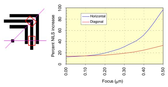
**Figure 8.** The improvement with square shape over circular, measured in terms of NILS increase, for horizontal and diagonal orientations.
