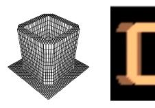
**Figure 13.** A square-ring annulus shape for off-axis illumination. This source is optimized for  $k_1$  near 0.40. Maximum overlap of diffraction orders is achieved, which is superior to circular-ring annular illumination.
